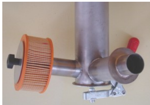
suction box with filter
