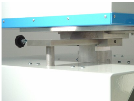
L-sliding guide different sizes for installation on different machines
