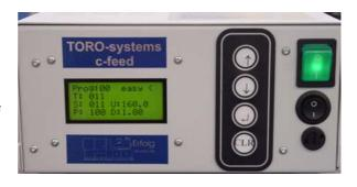
The connection to the processing machine can either be done with an extra connector for the dosing valve (advantage: the control unit gets the information when and how long the screw is rotating and can stop the injection moulding machine when the additive is empty) or a connector for the machine dosing signal (the information we get is depending on the machine signal).
