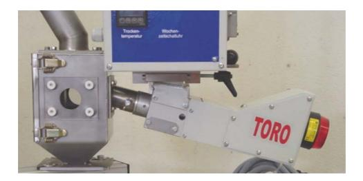
The MC control unit allows to store 98 different programs and is extremely easy to handle. To calibrate the **TORO-systems C-feed** (different additives need different calibration values) just fill up the hopper and press the calibration start button. The measured amount of additive during calibration, the shot weight and the percentage of additive is only entered into the MC control unit and every thing else is calculated by the MC control unit.
